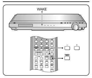
The SLEEP timer can turn the unit off after a set time and the WAKE timer can turn it on. You can use only one timer at a time.
